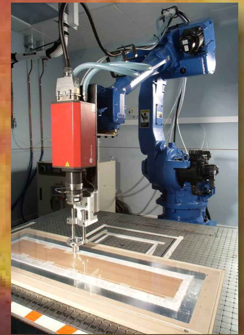
The ALTEX project aims to develop the fabric materials, equipment and procedures required to allow use of laser welding of seams in textiles
